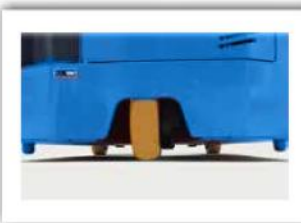
3-pivot design, with better stacking stability
